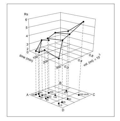
constant separation time, an increase in resolution could be observed. Going diagonally from D to B, i.e. increasing the gradient volume 2-fold while increasing the flow rate 4-fold, demonstrates how the separation time can be cut without losing resolution. As the resolution increases with increased gradient volume, however, dilution of each peak occurs, which also has to be taken into consideration.
