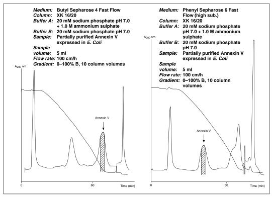
Fig. 9. Purification of Annexin V on Butyl Sepharose 4 Fast Flow and Phenyl Sepharose 6 Fast Flow (high sub). (Work from Amersham Pharmacia Biotech, Uppsala, Sweden).
