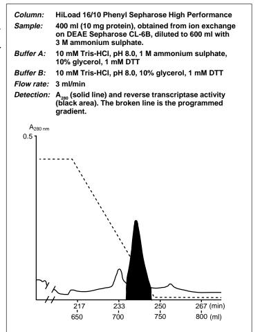
ammonium sulphate and applied to a column containing Phenyl Sepharose High Performance (Fig. 34). The HIC step was used both as a purification step and a concentration step and it reduced the volume 15 fold (from 600 to 40 ml). The final purification step was anion exchange with FPLC<sup>TM</sup> using a Mono Q<sup>TM</sup> column.
