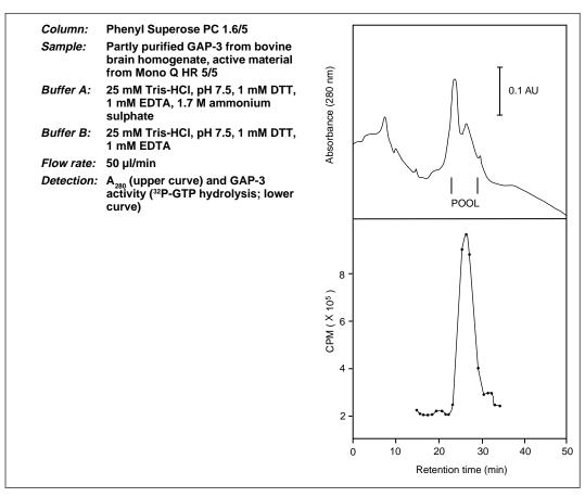
Fig. 36. Micropurification of GAP-3 (reproduced with permission, from ref. 52).
