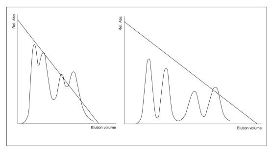
Fig. 19. Effect of gradient slope on resolution.
