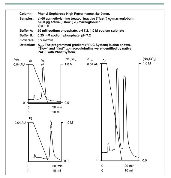
Fig. 39. Separation of conformational isomers of  $\alpha_{\!_2}\text{-macroglobulin}$  using HIC. (Work by Amersham Pharmacia Biotech).
