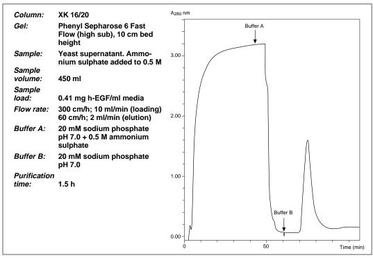
Fig. 45. Laboratory scale purification of h-EGF on Phenyl Sepharose 6 Fast Flow (high sub). (Work from Amersham Pharmacia Biotech, Uppsala, Sweden).
