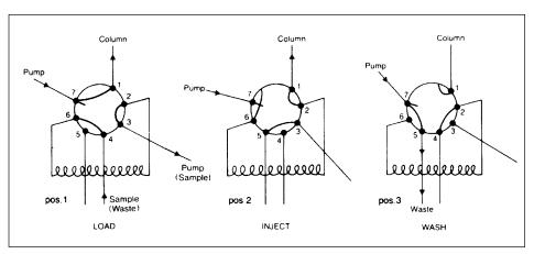
Fig. 28. Seven-port valves, V-7 and MV-7 have three operating positions which make sample application and changing eluents particularly convenient.
