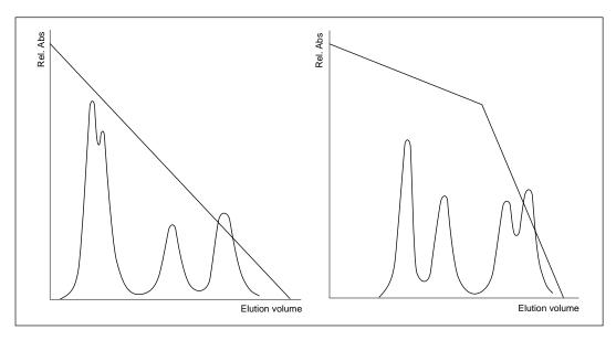
Fig. 18. Effect of a complex gradient on resolution.
