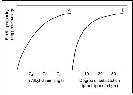
HIC media shown in Fig. 3 are all based on the glycidyl ether coupling procedure, which produces gels that are charge free and that should thus only have hydrophobic interactions with proteins. The phenyl group shown in Fig. 3-C also has a potential for b-b interactions. The glycidyl-ether coupling technique will introduce a short spacer but the effect of this will be very limited since the short hydrophobic chain is "neutralized" with the hydrophilic OH-group.
