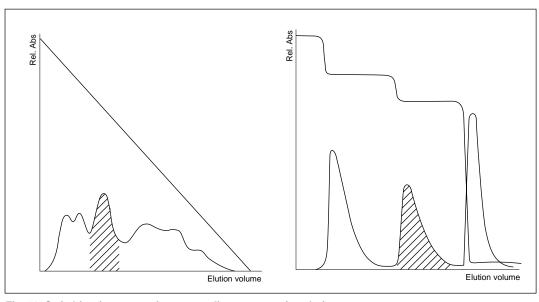
Fig. 20. Switching from a continuous gradient to step-wise elution.
