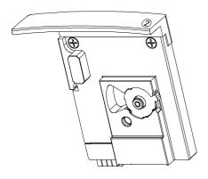
The pressure cartridge contains a tubing and filter assembly that connect to the vacuum pump. The seal has to match the priming well on the chip so that the required low pressure can be built up. The pressure cartridge can be identified by the engraved number "2" on the front.
