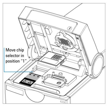
To avoid using incompatible chips and cartridges, a chip selector is installed in the bioanalyzer. This ensures that the chip matches to the installed cartridge.
