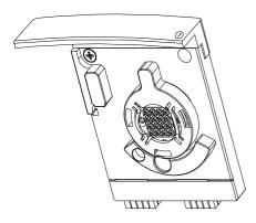
The electrode cartridge contains 16 electrodes that fit into the wells of DNA, RNA, and Protein chips. Each electrode in the cartridge has an individual power supply. All electrophoretic assays (DNA, RNA, and Protein) require an electrode cartridge. The electrode cartridges will either have an engraved "1" at the front, or will have no engraving at all. Cartridges with a different number are not electrode cartridges.
